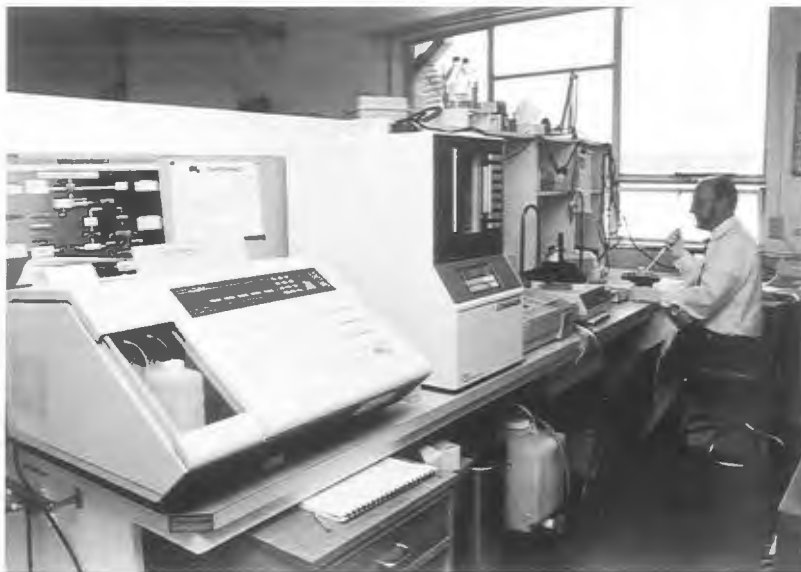
Automated Immunology (1990's), E.I.A (Abbott IMX), Incubator, Spectrophotometer (Quantum II) and Quickwash Unit.
